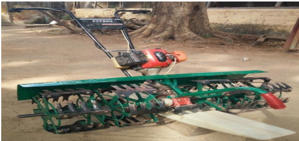
Fig. 3.30. Power operated 8-row drum seeder cum 4-row weeder for paddy
