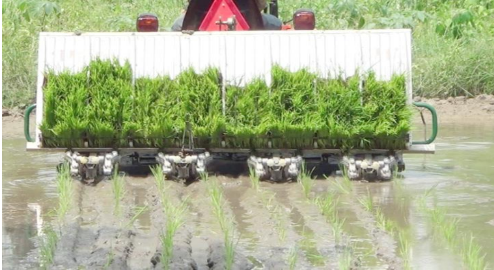
Fig. 3.29. Four wheel drive tractor mounted 8-row paddy transplanter
