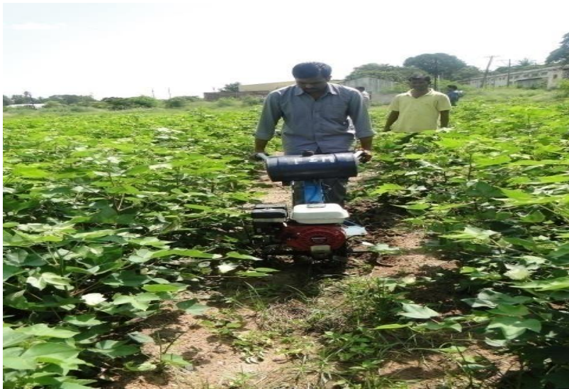
Fig. 3.31. Stem applicator cum weeder in cotton
