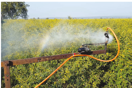
Insecticide spraying with a boom sprayer mounted on a baby tractor
